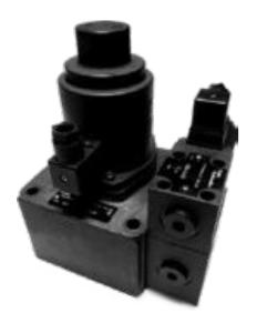
EBDG series proportional pressure and flow control valves adopt two electrical loops to control pressure and flow of hydraulic system respectively. Using very small pressure drop to track load pressure and control the pump pressure, it is an energy-saving valve.
