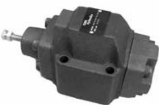
H(C)G series sequence counter balance unloading valves can be used as sequence valve, counter balance valve or unloading valve by different assembly. C type is with a check valve.
